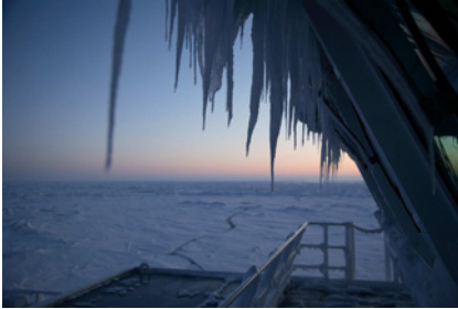
Figure 5.7: Danger posed by falling ice (Courtesy ©Arno Keinonen)
