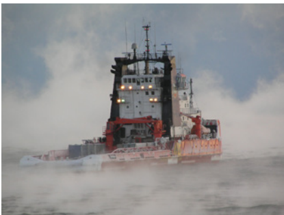
Figure 4.3: Icebreaking offshore support vessel
