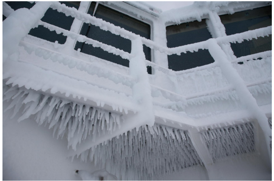
Figure 1.1: Ice accretion (Courtesy @Arno Keinonen)
