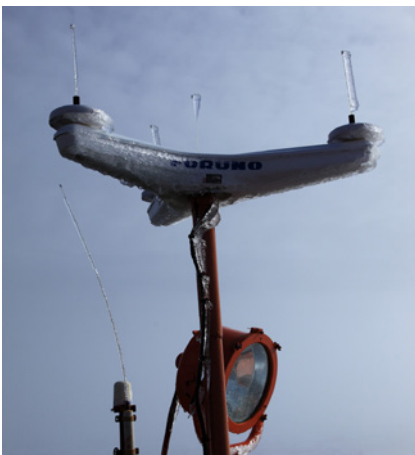
Figure 4.2: Icing on antennas
