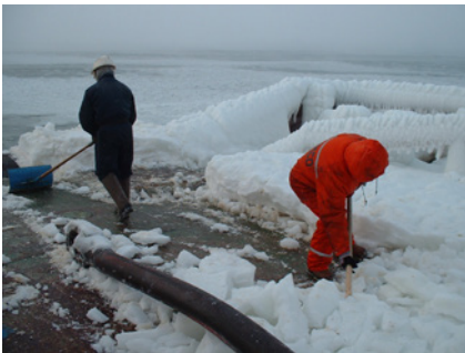
Figure 5.4: Ice accretion on deck
