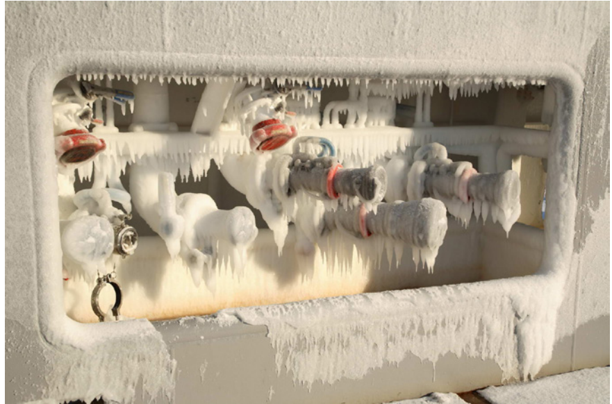
Figure 5.3: Ice accretion on supply boat manifold
