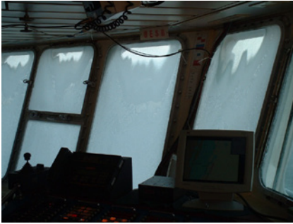
Figure 4.1: The effect of inadequate heating for wheelhouse windows
