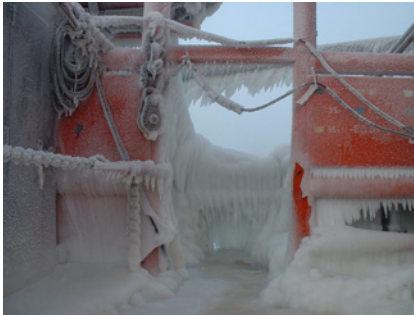
Figure 5.5: Ice accretion on deck passageways
