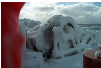
Figure 5.6: Ice accretion on deck machinery
